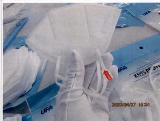
† 27 - Dirty mark on unit surface
