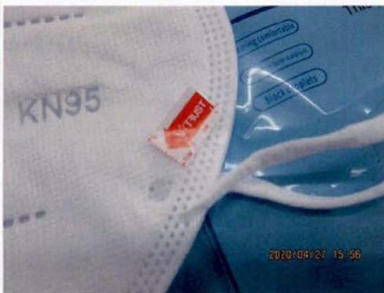
† 25 - Broken connecting rope
