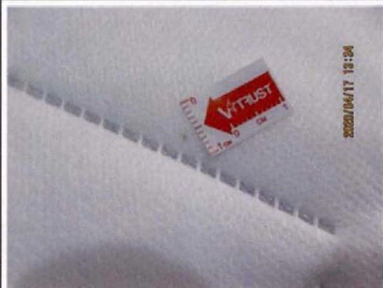
† 22 - Slight dirt stains on unit - minor
