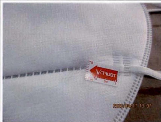
† 25 - Slight dirt stains on unit - minor
