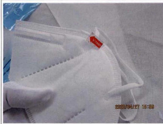
† 41 - Poor cutting on edge
