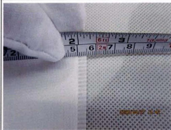
† 6 - Remark 2: 180PCS out of 500PCS, the width of the edge was uneven.
