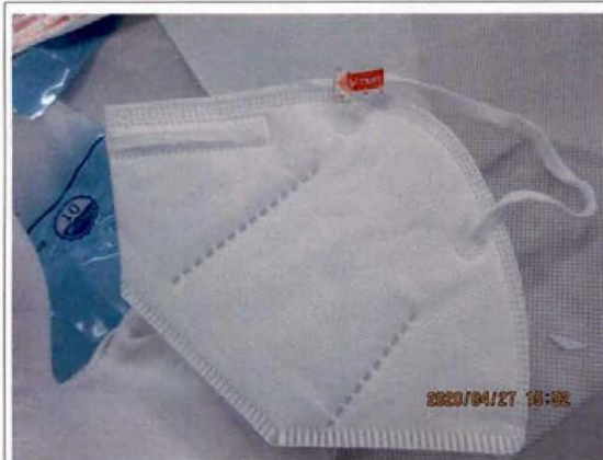
† 39 - Poor cutting on edge
