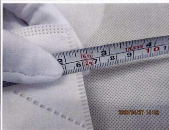
† 5 - Remark 2: 180PCS out of 500PCS, the width of the edge was uneven.
