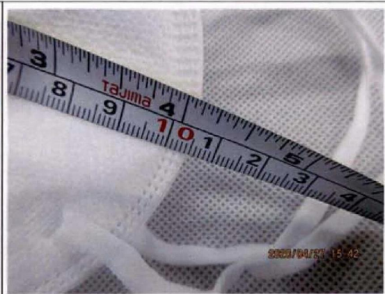
† 2 - Remark 2: 180PCS out of 500PCS, the width of the edge was uneven.
