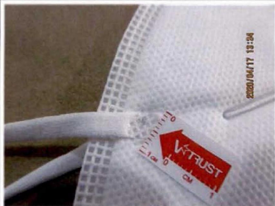
† 21 - Slight dirt stains on unit - minor
