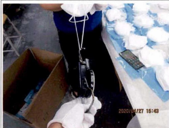
† 17 - Remark 7: The mask rope would detach from body when pull it with 6-7N force. It should be 10N force without breaking for standard.
