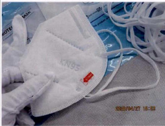
† 23 - Broken connecting rope
