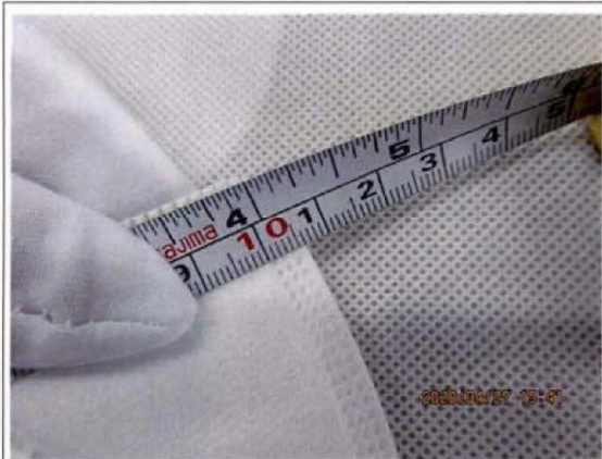
† 1 - Remark 2: 180PCS out of 500PCS, the width of the edge was uneven.
