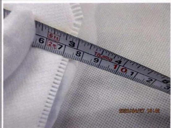
† 4 - Remark 2: 180PCS out of 500PCS, the width of the edge was uneven.
