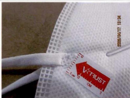
† 21 - Slight dirt stains on unit - minor
