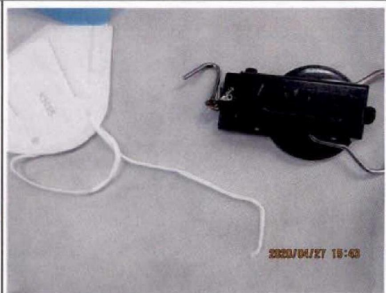
† 18 - Remark 7: The mask rope would detach from body when pull it with 6-7N force. It should be 10N force without breaking for standard.
