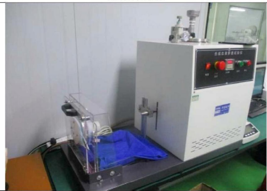
Synthetic blood penetration test
