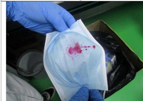
Synthetic blood penetration test
