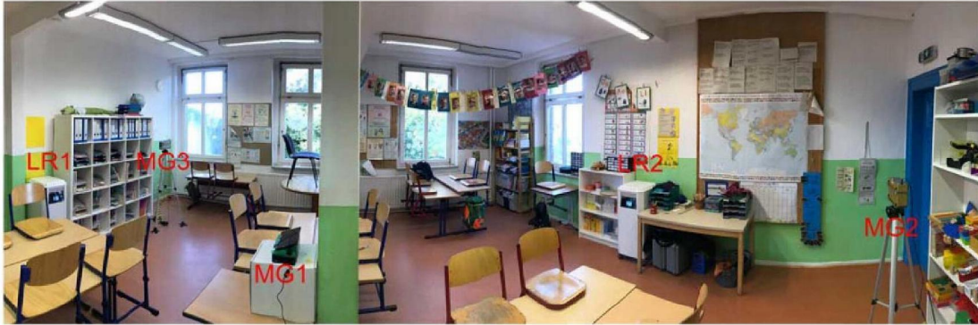
Fig. 1: Panorama photo of the tested classroom (L x W x H: 7 m x 6.7 m x 3 m) with measuring devices (MG/Messgerät) and air purifiers (LR/Luftreiniger)
