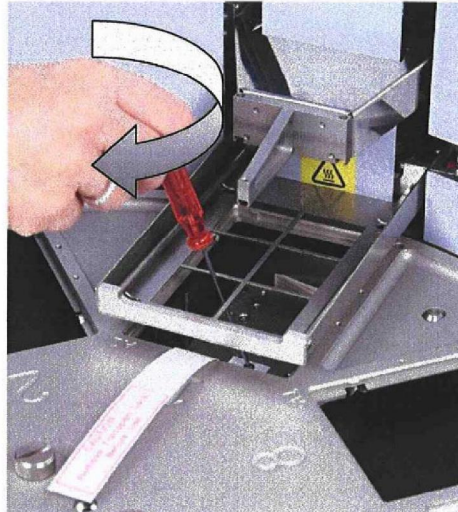
Figure 3–27. Refitting the transport lock of the heating block (B)
