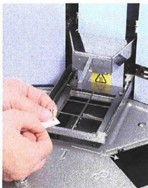
Figure 26 Refitting the transport lock of the heating block (A)
