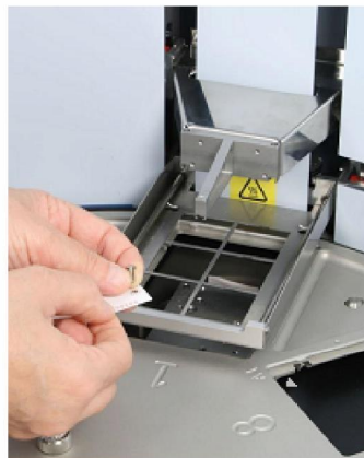
Figure 3-26. Refitting the transport lock of the heating block (A)
