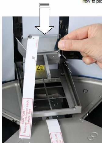
Figure 3-28. Fitting the transport lock of the tip comb holder (A)
