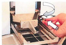
Figure 30 Fitting the transport lock of the tip comb holder
