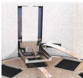
Figure 31 Both transport locks refitted
