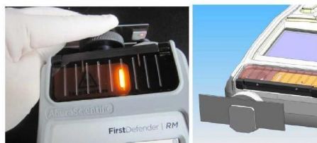
Figure 1 Handheld Raman system integrated with AgNR array substrates: Left: with a handheld substrate; Right: with a special substrate holder.
