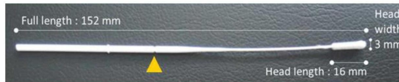
Figure 16: Unpacked sterilized nasopharyngeal swab, Noble Biosciences. Breakpoint is indicated by a yellow triangle.
