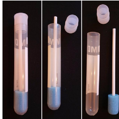
Figure 2. The sponge in the tube and when removed from the tube. Keep the cap clean. After oral fluid has been collected the sponge is put back in the tube in reverse order.
